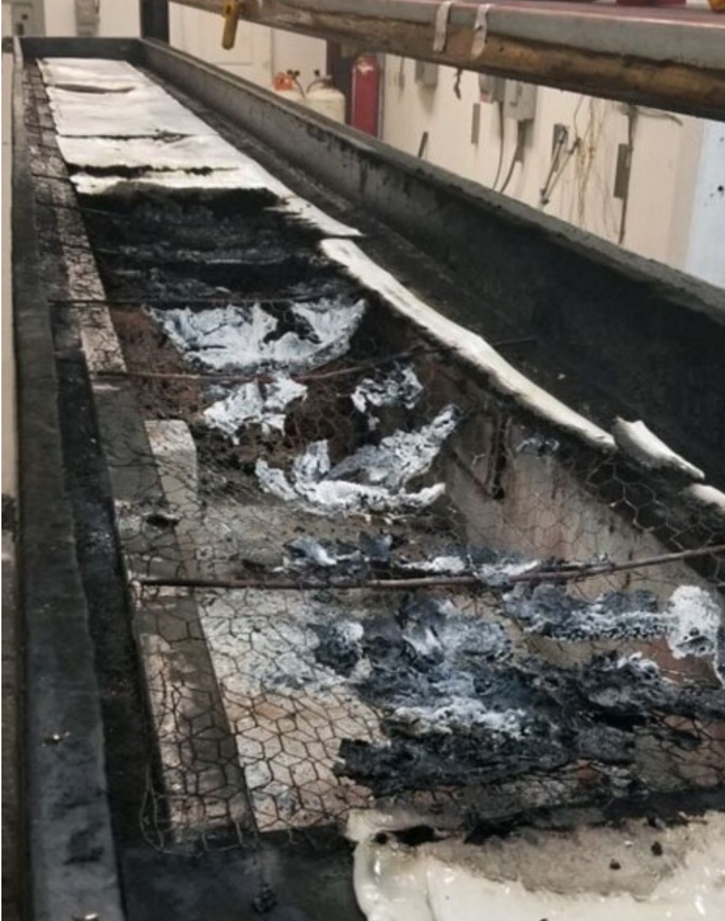
Photograph No. 2: The test specimen after the 10-minute fire exposure test shown from the chamber's burner end.
